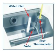
Rudolph provides a temperature validation cell with every TempTrol<sup>TM</sup> system. The temperature validation cell along with an optional NIST traceable thermometer is designed to validate the temperature control performance of the polarimeter and cell to ±0.2°C.
