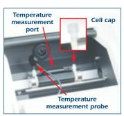
For improved temperature performance or when working with acids (HCl) use the measurement port in the body of the cell. This also allows the inlet and outlet ports to be capped to avoid evaporation, fumes and spillage.
