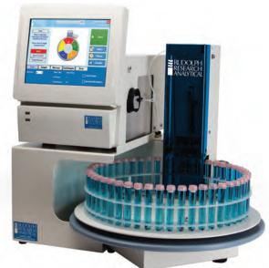
Operation is completely automatic. The sample is measured and the data recorded. Depending on how the system is configured the data may also be printed, saved as an Excel file or transferred to a LIMS system.
