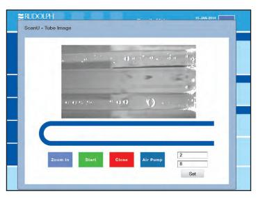
A full view of the entire U-tube is possible without any obstruction. Automatic Scanning of U-tube under the 10X magnification of the entire U-tube and manual control is possible to view any position of the U-tube. The clarity, magnification and resolution is the very best available. Rudolph's exclusive VideoView is protected under Patent #7,437,909.
