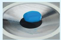
A small drop of sample in the center of the prism will measure correctly. A large drop of sample completely covering the prism surface will measure correctly. A small drop on the perimeter of the prism will produce erroneous results.
